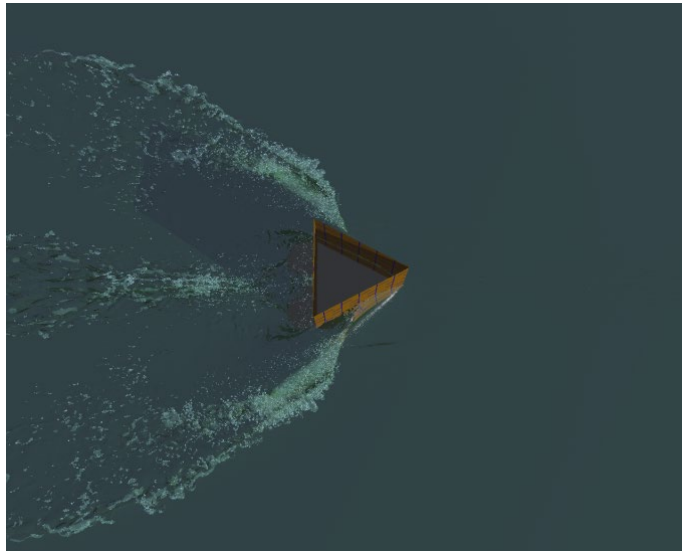
Figure 1. Wave breaking around a wedge-shaped bow.
