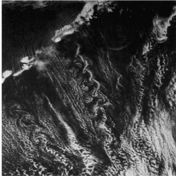
FIGURE 9.19 A von Karman vortex street downstream of mountain peaks in a strongly stratified atmosphere. There are several mountain peaks along the linear, light-colored feature running diagonally in the upper left-hand corner of the photograph. North is upward, and the wind is blowing toward the southeast. R. E. Thomson and J. F. R. Gower, Monthly Weather Review 105: 873–884, 1977; reprinted with the permission of the American Meteorological Society.
