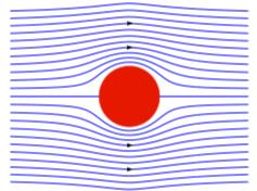
Streamlines for the incompressible potential flow around a circular cylinder in a uniform onflow.
