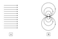
A potential flow is constructed by adding simple elementary flows and observing the result.
