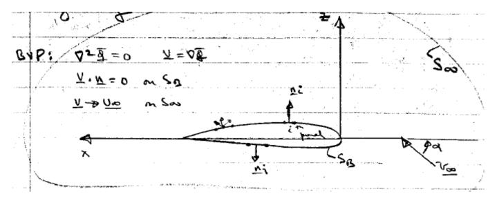
$$\frac{DF}{Dt} = 0 \rightarrow \frac{\partial F}{\partial t} + \underline{V}. \nabla F = 0 \rightarrow \underline{V}.\underline{n} = -\frac{1}{|\nabla F|} \frac{\partial F}{\partial t}$$
