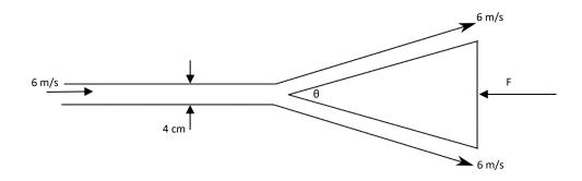
Continuity equation:  $-\frac{d}{dt}\int_{CV}\rho d\forall = \int_{CS}\rho\underline{V_R}\cdot\underline{n}dA$  Momentum equation:  $\sum F = \frac{d}{dt}\int_{CV}\rho\underline{V}d\forall + \int_{CS}\rho\underline{V}\underline{V_R}\cdot\underline{n}dA$
