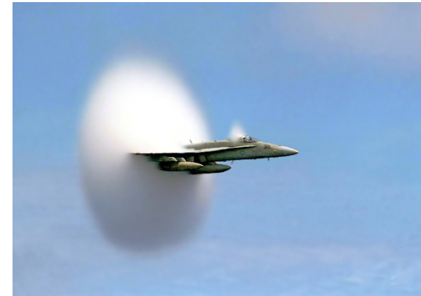
U.S. Navy F/A-18 approaching the sound barrier. The white cloud forms as a result of the supersonic expansion fans dropping the air temperature below the dew point.
