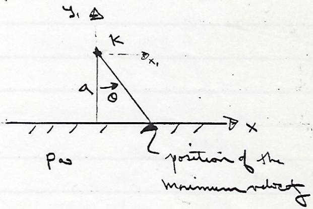
$$\begin{aligned}\Phi &= \alpha_1 + \alpha_2 \quad \text{where } \alpha_2 \text{ is the image} \\ &= \frac{K}{2\pi} \left[ \ln \sqrt{x^2 + (y+a)^2} + \ln \sqrt{x^2 + (y-a)^2} \right]\end{aligned}$$
