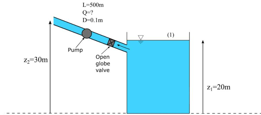
$$\text{Energy equation } \left( \frac{P}{\rho g} + \frac{V^2}{2g} + z \right)_1 = \left( \frac{P}{\rho g} + \frac{V^2}{2g} + z \right)_2 + h_f + h_t - h_p$$
