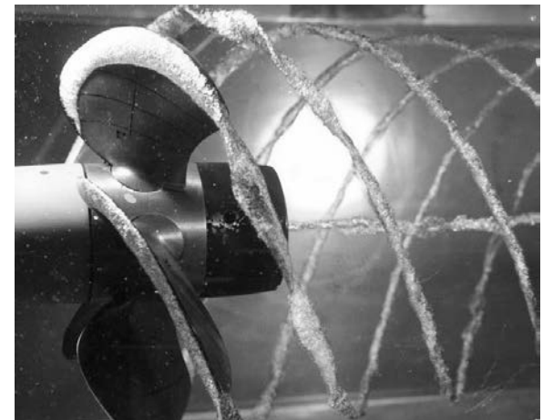
Cavitation formed on a marine propeller
