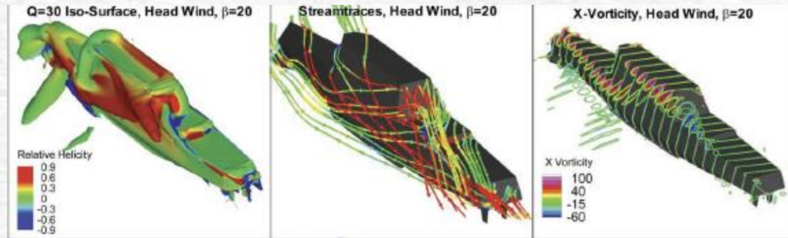
Air flow for ONR Tumblehome in Planar motion mechanism (PMM) maneuvers
