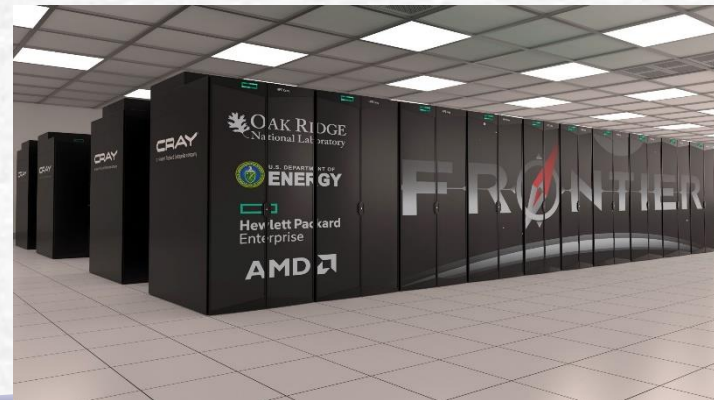
Supercomputer FRONTIER, DOE/SC/Oak Ridge National Laboratory, Peak Compute: 1,679.82 (PFlop/s), TOP500: 1st, June 2022-2024
